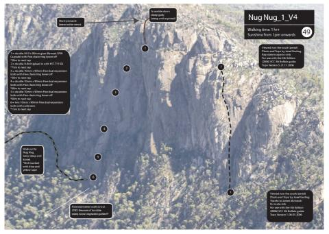
Refer to the cliff topo (aerial photo) showing the approximate position of the abseil stations. Please note that another rap station is required between 2& 3 to get down with two 60m ropes (this abseil is currently approx 75m). Two 60m ropes are required for about half the abseils. The abseil stations are all modern stainless steel, with a mixture of expansion and chemical anchors used.
